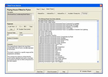
Figure 3 – SAS Beta 1.1 – Risk Threat Module for 6 kg Training Bomb showing some of the summary of the threats during the Flying Hours Fitted to Pylon phase.
